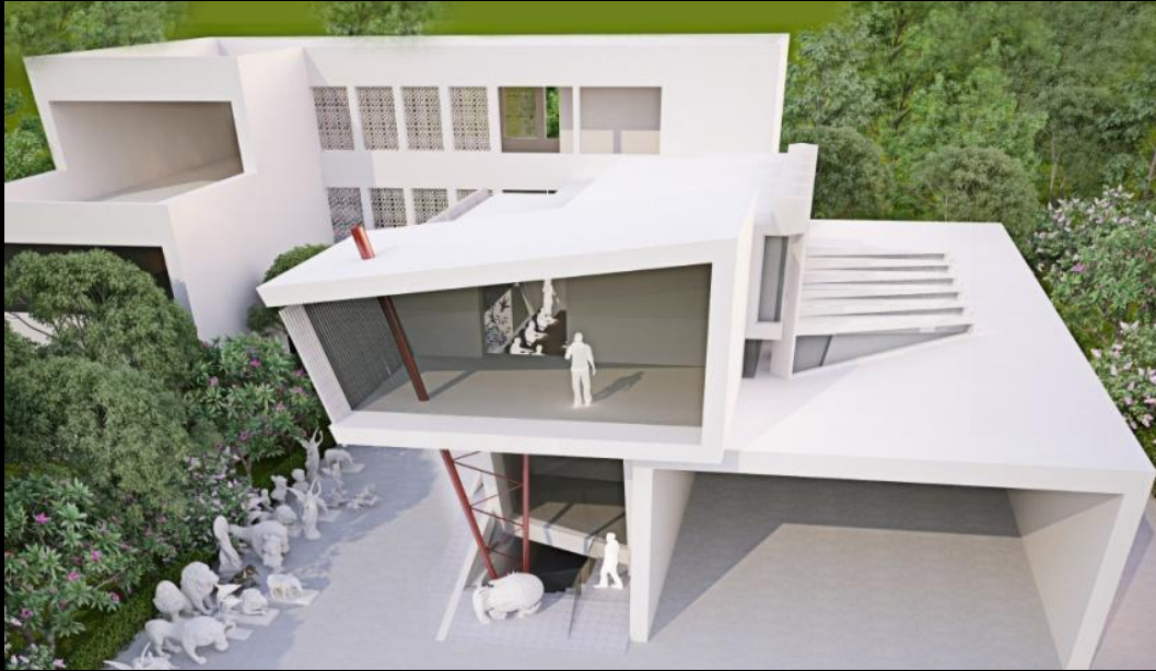
DISPLACEMENT OF BLOCKS TO GET NATURAL LIGHT INTO THE BASEMENT AND UPPER FLOORS OF THE BUILDING.
